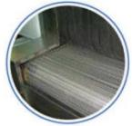
The conveyor belt is made of a strong stainless chain with open cells of at least 15x15 mm and has additional supports - rollers, which allows to withstand a load of not less than 100 kg per meter of conveyor length. The conveyor is driven by a worm gear motor and has a tensioning station. The conveyor speed can be adjusted in the range of 1-6 m / min.
